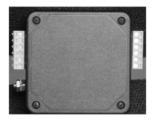
Low speed ST-CLMFxx-y [z = blank (2 Mbps.)] series models are designed to protect current loop circuits, signal lines &/or slow-speed data lines feeding transducers, leak detectors, flow meters and a broad variety of similar sensory devices. High-speed data signal lines and equipment may be protected using the ST-CLMFxx-yX [z = X (10 Mbps)] or the ST-CLMFxx-yC [z = C (100 Mbps)]. \*Models may be optioned with 2, 4 or 6 terminal connections as shown above.
